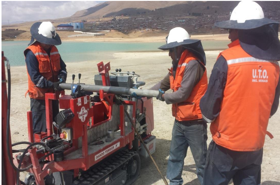
Figure 3. Removing the sample from the drill core at Kenko.
