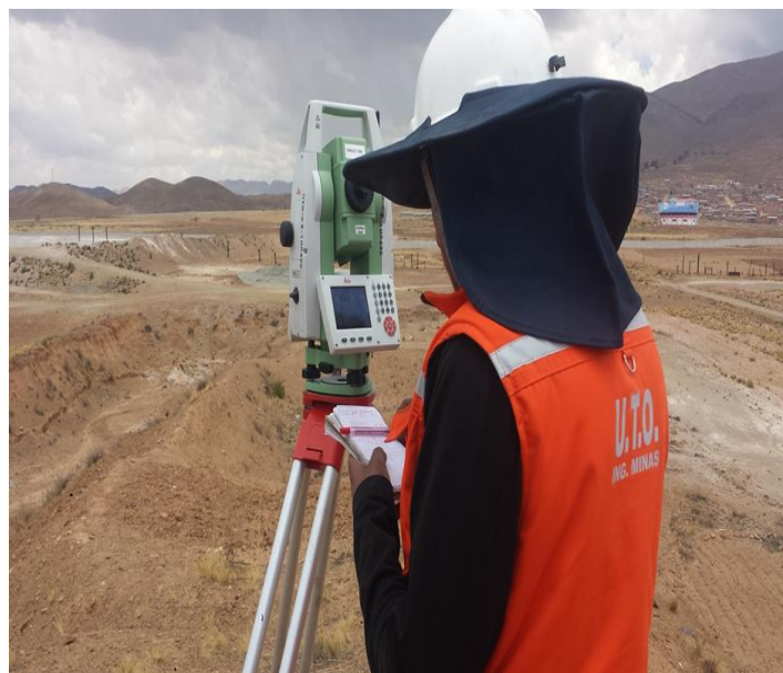
Figure 7. LEICA TS-09 from Leica Geosystems being used for Kenko survey
