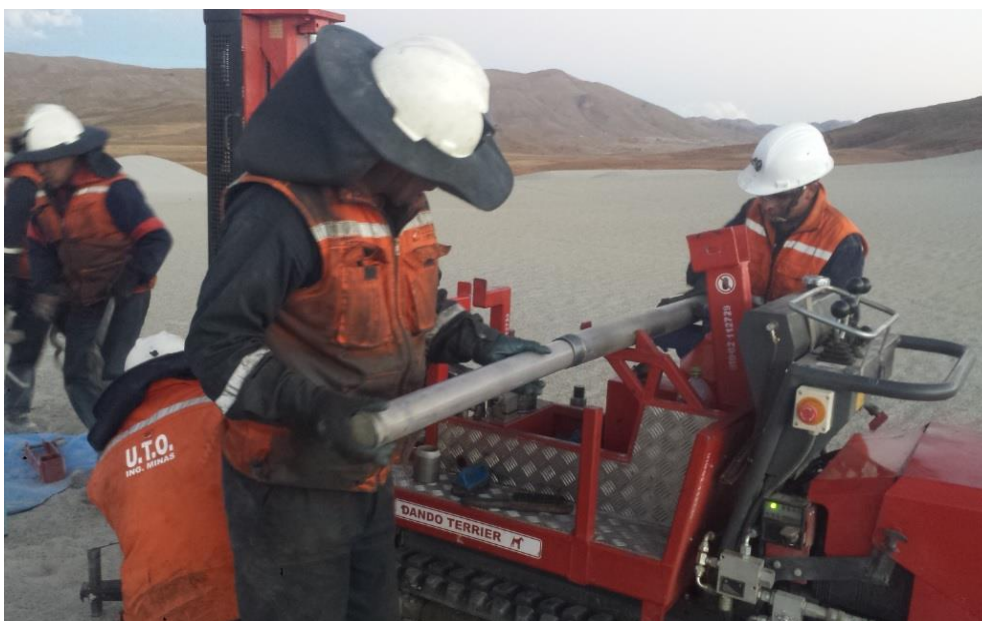
Figure 4. Taking out the sample from the drill core at Arenas Catavi
